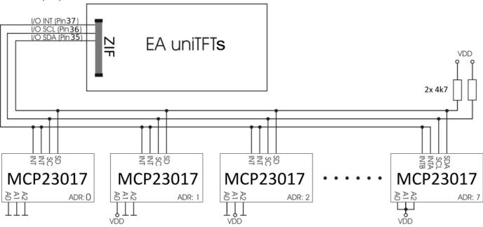
The maximum power of the MCP23017-E is 700 mW in total. The maximum current load for a single pin is 25 mA, which makes it possible to directly operate a low current LED. If a higher load is required, the I/O current must be amplified with suitable circuitry, e.g. through an external transistor. For more details see <u>Electrical characteristics</u>
