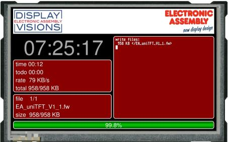
After transferring the data, a manually reset needs to be performed, then the firmware will be loaded automatically
