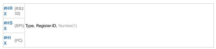
The command sends a Number of register entries (Register-ID) in binary form via the master interface.
