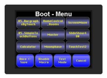
To avoid mis-use by the operator, the boot menu can be deactivated. For this purpose, an empty file named "bootmenu.off" must be placed in the root directory of the memory. This can be done using mass storage mode and Windows Explorer to transfer the file, or directly via uniTFTs commands:
