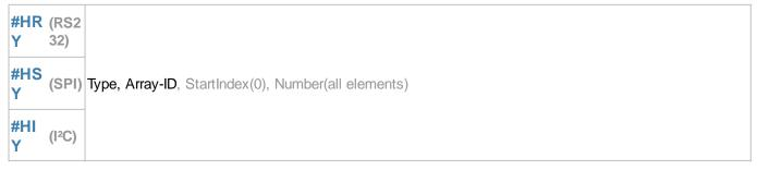
The command sends a **Number** of array elements (**Array-ID**), starting with the start index, in binary form via the master interface.
