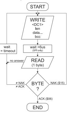
The user data is transferred framed by <DC1>, the number of bytes (len) and the checksum (bcc). The display responds with <ACK>.
