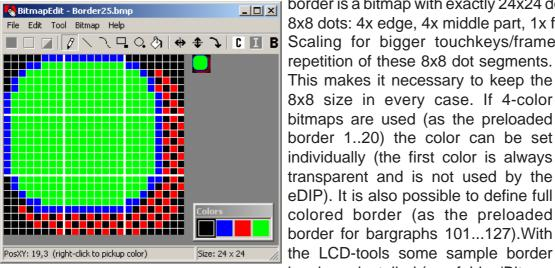
border is a bitmap with exactly 24x24 dots (9 segments with 8x8 dots: 4x edge, 4x middle part, 1x filling).
