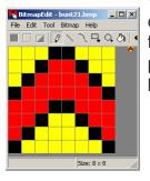
With the LCD-tools it is possible to define new pattern (=bitmaps with exactly 8x8 dots).(Compileroption "Pattern:"). The foreground- and backgound color can be set for monochrome pattern (as the 20 preloaded pattern) incl. transparency. It is also possible to define full colored pattern. With the LCD-tools some sample pattern has been installed (see folder 'Pattern').
