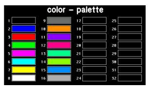
number between 1..32. The dummy color number 255 means that the actually color is not changed e.g you want only to change the foreground- and not the background color. The color number 0=transparent is special and can be used for background of character e.g. that means that for placing a character no rectangular field will be deleted around the character itself. The sensless combination
