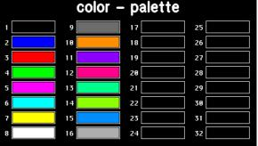
between 1..32. The dummy color number 255 means that the actually color is not changed e.g you want only to change the foreground- and not the background color. The color number 0=transparent is special and can be used for background of character e.g. that means that for placing a character no rectangular field will be deleted around the character itself. The sensless combination of transparent
