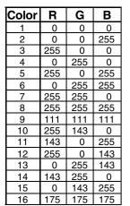
redefined at any time without changing the content of the display (command: ESC FP no R G B). To use a color for text and graphic functions you set only a number
