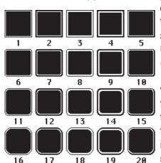
commands draw box frame and draw touchkeys. There are also three special borders in various colors for using with bargraph commands (no:101..107, 111..117 121..127). All of them can be used in various sizes via coordinates. The frames 1..20 are split into 3 segments: the outer frame, inner frame and filling. Each segment will get an individual colour for normal and for selected state. This will give the user
