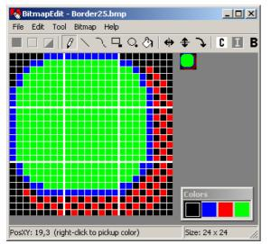
Scaling for bigger touchkeys/ frames will be done by repetition of these 8x8 dot segments. This makes it necessary to keep the 8x8 size in every case. If 4-color bitmaps are used (as the preloaded border 1..20) the color can be set individually (the first color is always transparent and is not used by the eDIP). It is also possible to define full colored border (as the
