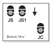
**Important:** Always place all solder straps in the same position and desolder them cleanly. Short circuits destroy the eDIP320-8.
