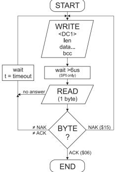
The user data is transferred framed by <DC1>, the number of bytes (len) and the checksum (bcc). The display responds with <ACK>.
