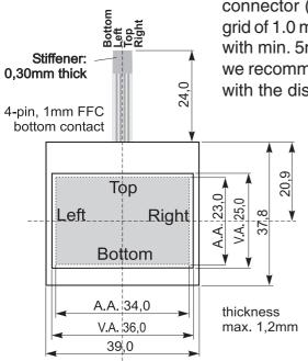
connector (e.g. EA WF100-04S) with a grid of 1.0 mm. Bending radius is defined with min. 5mm. For optimum readability we recommend that you use a backlight with the display.
