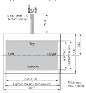
EA WF100-04S) with a grid of 1.0 mm. Bending radius is defined with min. 5mm. For optimum readability we recommend that you
