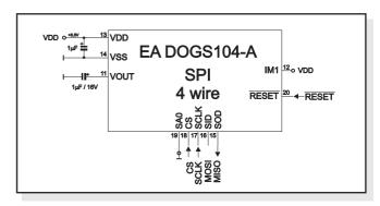
To guarantee an error-free functionality and initialization of display it is recommended to operate the reset input actively. This can be done via microcontroller port or external circuit. Here's an application
