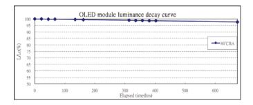
operated 100,000 hours and more at room temperature. Even when used at maximum operating temperature (80°C), they retain 50 percent or their original brightness after 14,000 hours.
