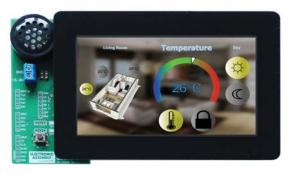
even be operated with a pencil or gloves; The PCAP version performs even behind a 4 mm thick glass or with thin gloves and is multitouch-capable.
