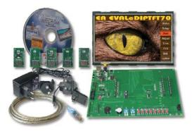
Integration of the intelligent display into a device or system controller is very easy from the technical standpoint. Three different ports are available for communication with the system. Only one supply voltage is needed. A mounting bezel is available as an option.
