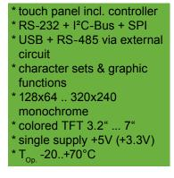
three different interfaces – RS 232, I<sup>2</sup>C bus, and SPI bus. The display can be used in an enhanced temperature range of -20°C to +70°C.
