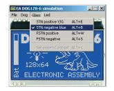
background illumination schemes translates into a total of 63 "customization" options for character displays and there are a lot more graphic types also. Two or three separate LED paths are available for the unicolor backlights, so the illumination unit can therefore be operated using a 3.3 V or a 5 V power supply.
