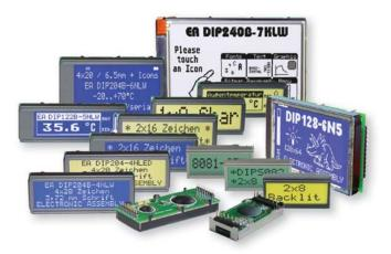
ELECTRONIC ASSEMBLY has designed the EA DIP162-DN3LW LCD module for applications where the display has to be clearly legible. The module comes with a high-contrast alphanumeric LCD supertwist display for showing two 16-character lines. LED background lighting supplied as a standard feature makes the text clearly stand out.
