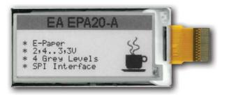
Thanks to the integrated battery (CR2032) the EA ELABEL20-A may be plugged-off from pc after pictures and text are loaded. Demos run automatically. Switching off the battery freezes the display content. Forever.
