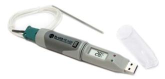
seconds to 12 hours to customize the monitoring period, which can span as little as 5 hours or as much as 1 year. The time at which measurements are to be taken is also programmable.
